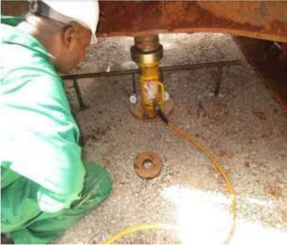
Plates 4&5: Taking the dial gauge readings after applying the loads
